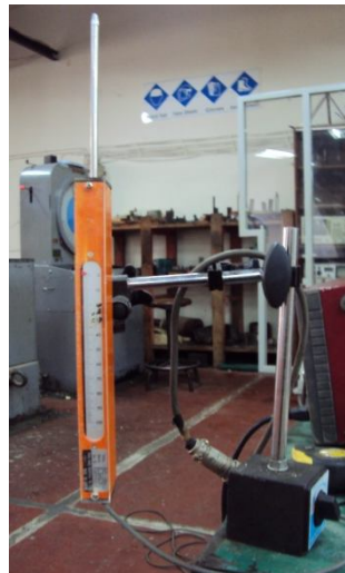
Gambar 6. 2 linear variable differential transformer (LVDT)
