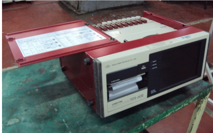
Gambar 6. 3 Computing data logger TDS-602
