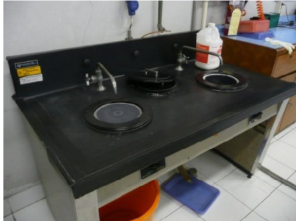
Gambar 3.5 Mesin grinding dan polishing tipe Buehler Polisher (10)
