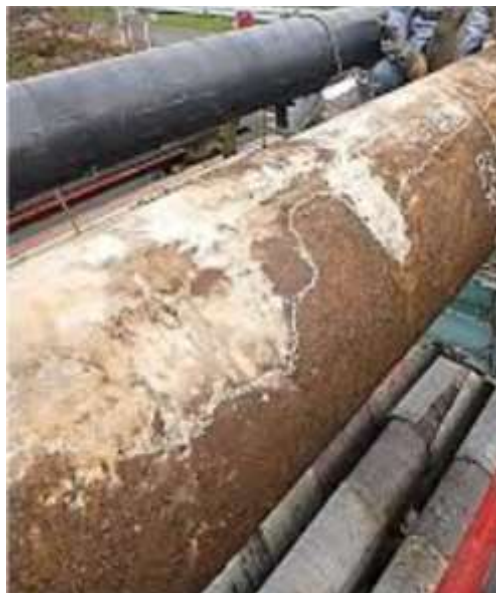
Gambar 2.17 Ilustrasi korosi general [3]
