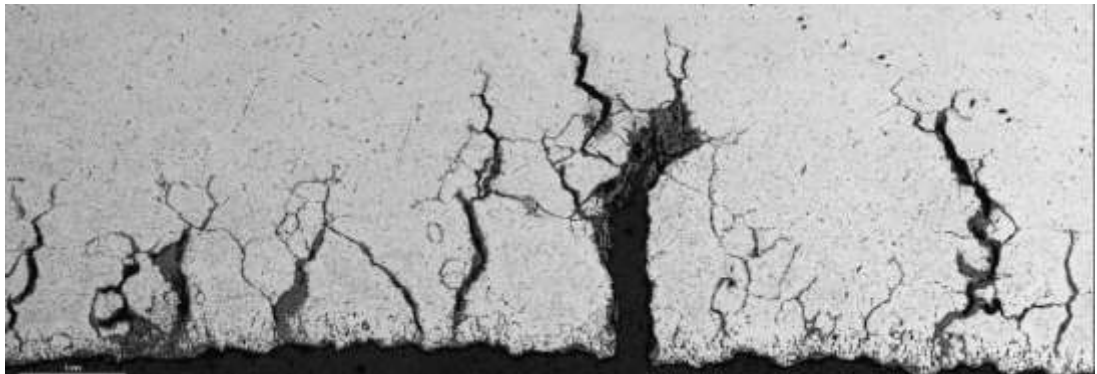
Gambar 2.20 Ilustrasi stress corrosion cracking [14]
